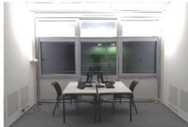
Figure 1. The lab room seen from the inside. The light-emitting structures are placed on the top part of the windows and provide illumination to the room interior.
