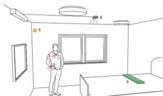
Figure 5. Devices used for monitoring over a period of two weeks in November 2019. 1) and 2) wearables, 3) mobility monitor, 4) camera sensor, 5) temperature sensor.
