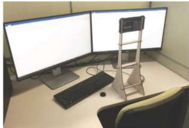
Fig. 4. Assessment of the luminous environment and glare sources using a mobile device and micro fish-eye lens.
