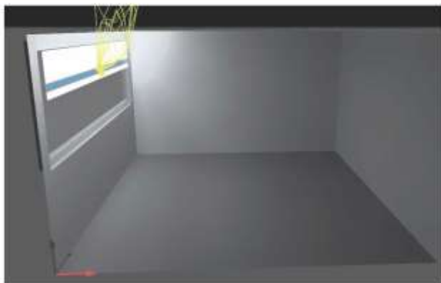
Figure 6. Dialux rendering of the light-emitting structure used in this case study.
