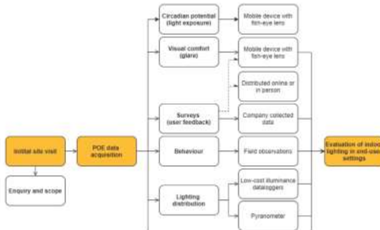
Figure 3. Post-occupancy (POE) framework to collect objective and subjective measures of the indoor lighting environment specific to occupied end-user settings in large open plan office environments.
