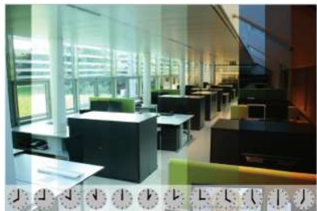
Figure 1. Careful daylighting design is integrated with CCT tuning at the Bartenbach headquarter in Aldrans, Austria.
