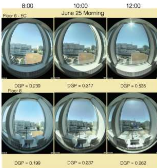
Figure 7. Discomfort glare levels in EC office (above) versus reference office (below) on a sunny day. Glare levels in the EC office were "intolerable" at noon due to the sun in the field of view. EC set to Tint 1.
