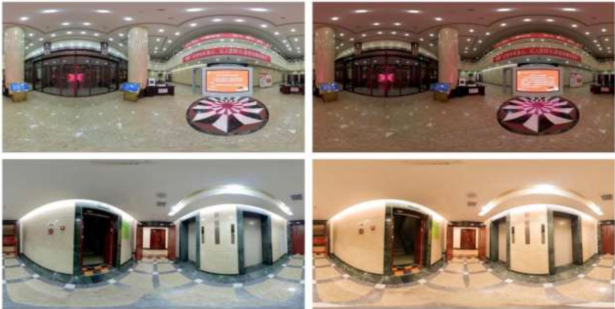
Figure 4. Details of two of the common areas in the building. The extreme CCT settings are shown in picture.
