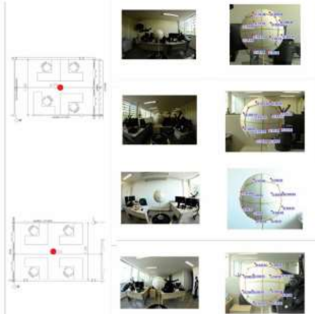
Figure 7. HDR photographs of the sphere to calculate daylight directionality in Room 1 – South (top) and Room 2 - North (bottom).
