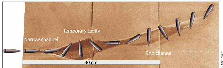
Figure 3.14 The bullet tumbles in the gelatine or soap: it rotates 270° around a transverse axis that is perpendicular to the long axis. (Graphic demonstration of bullet superimposed on soap blocks. The proportions between bullet and trajectory are exaggerated for the sake of clarity.)
