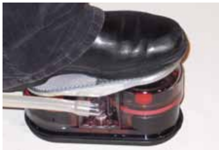
Figure 17.1.3 Foot-driven suction pump.
