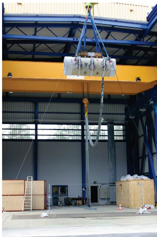
Figure G-1: Drop test of a transport and storage cask for vitrified waste at the test facility of the Federal Institute for Materials Research and Testing (BAM) within the framework of an approval procedure under traffic law (Copyright: BAM)
