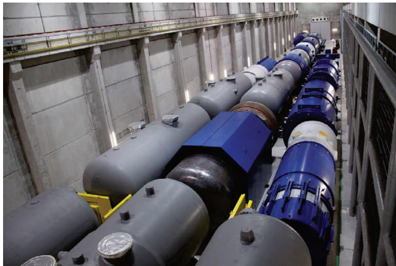
Figure D-8: Decay storage of large components (steam generator, reactor pressure vessel) at the Zwischenlager Nord (ZLN) (Copyright: EWN)
