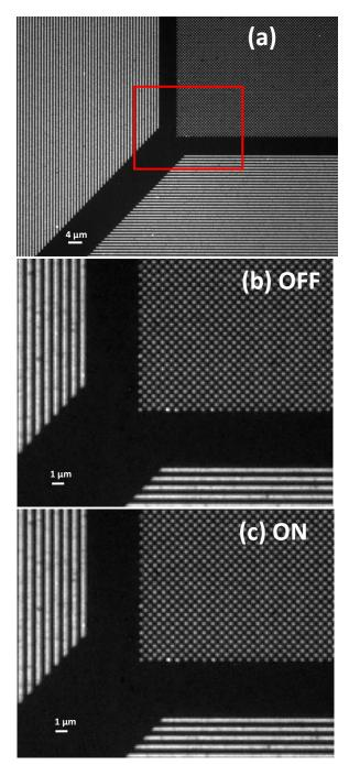
Figure 3: Sequence of images acquired with a wide-field microscope on the attoDRY800: 400 nm pattern (a) full image showing area (indicated by red square) used to demonstrate difference between cryostat (b) OFF and (c) ON.
