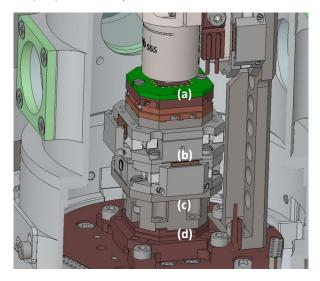
Figure 2: Details of the stack of the LT-APO configuration.
