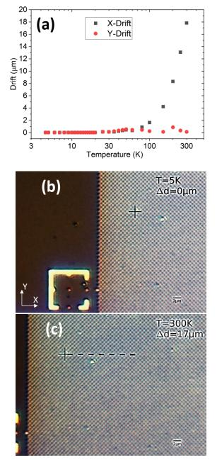
Figure 5: Lateral drift of target: (a) Drift in two lateral direction with respect to objective as function of temperature. Enlarged image of 500 nm checkerboard pattern at (b) 5 K and (c) 300K. The cross mark indicates the defect square, from which we measured the drift of the center of the image. The dashed line is between cross mark at 300K and center of the image.
