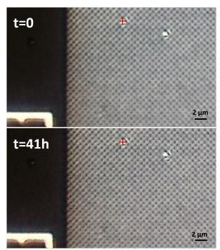
Figure 4: LT-APO image at 3.9 K of a 500 nm checkerboard pattern demonstrating time stability: top image acquired at t=0 and bottom image acquired in the very same conditions at t=41 hours without changing any measurement condition. The cross marker did not move within the resolution. Thus, we can remark a completely negligible drift of the image, i.e. less than one pixel size (53.5 nm).
