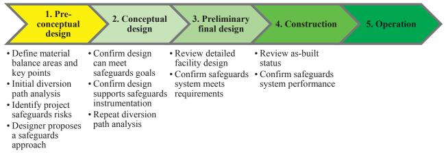
FIG. 1. Safeguards by design implementation during facility design stages (adapted from Ref. [12]).
