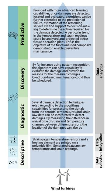
Figure 6: Smart composite for wind turbine safe and efficient operations
