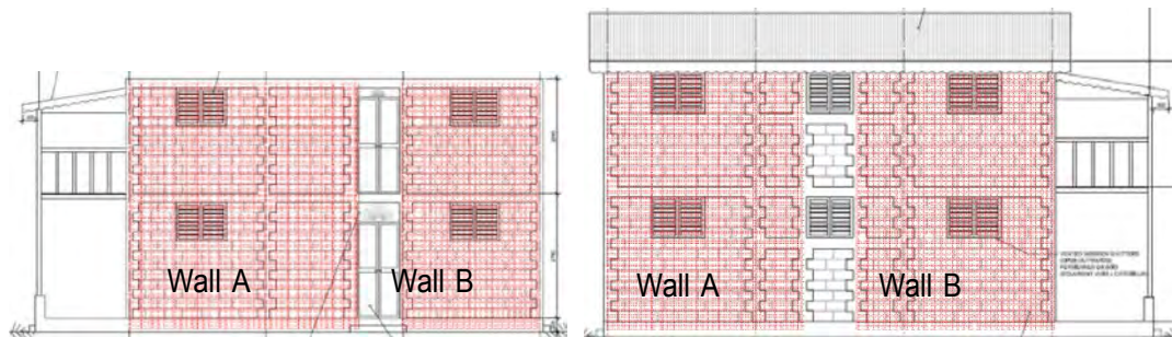
Figure 3.1 Examples of subdivision of walls into individual shear walls (each bounded by tie columns with at most one opening) for in-plane shear calculations
