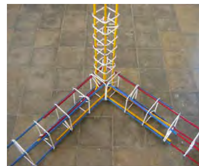
Figure 3. Bond Beam-Tie Column Connection Model. Note it has been suggested that to strengthen the interior corner, the interior long bars should pass through the joint and tie to the external long bars.
