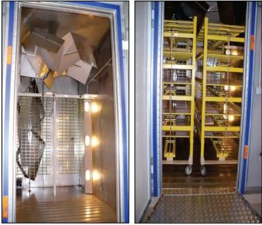
FIGURE 3 Exterior view of chambers, empty chamber showing the vertical and horizontal stirrers, and chamber with cage racks in place
