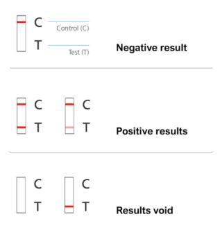
Image showing the results a lateral flow test might show
