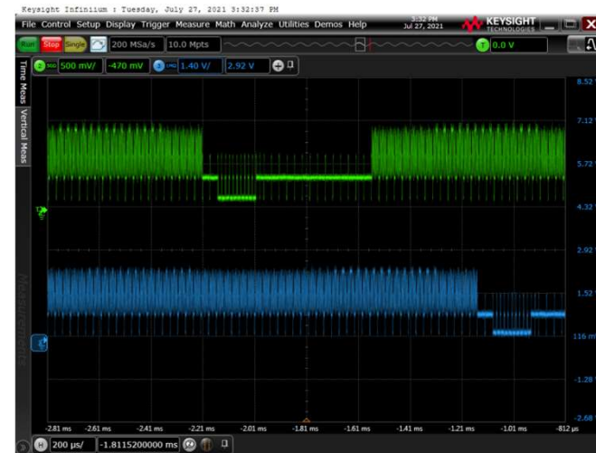
Video buffer set to 20 packets: transceiver to receiver latency 1.06 ms
