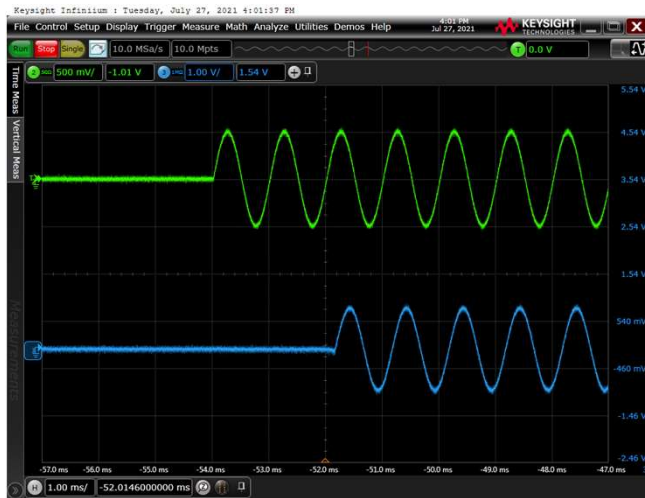
Audio buffer set to 32 samples: transceiver to receiver latency 2.2 ms
