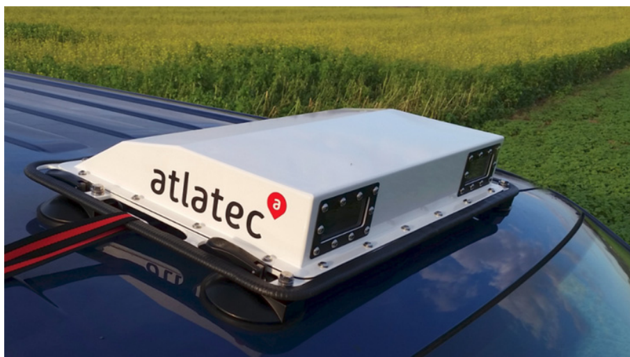
Figure 30: Atlatec's data collection platform is simply two cameras mounted on top of a vehicle (source: e-mail correspondence with Atlatec).
