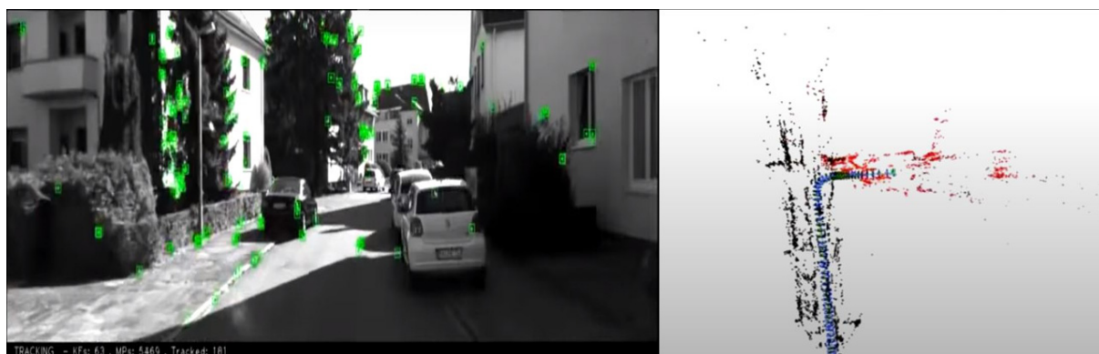
Figure 5: ORB-SLAM in action, detecting visual features in the left and producing keyframes on the right [20].
