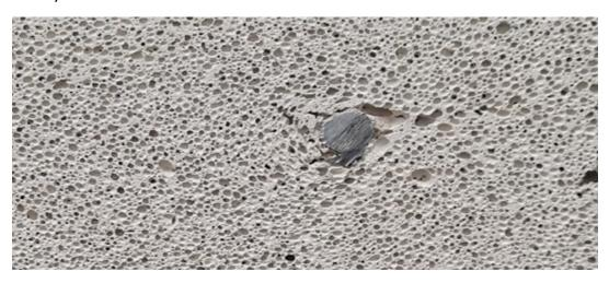
As a result, RAAC is weaker that standard density concrete, and more prone to damage from water and vibration. RAAC was intended to have a 30-40 year lifespan, but as successive Governments have failed to build enough new school buildings, its usage has extended to the point where critical failure is a realistic possibility.
