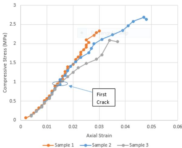
Fig. 21. Compressive stress vs Axial stress
