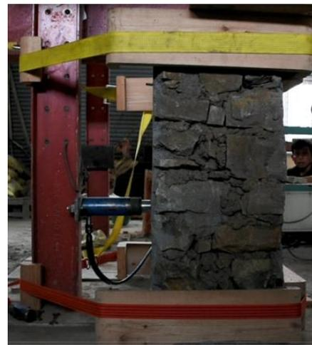
Fig. 23. dowel push out tests setup
