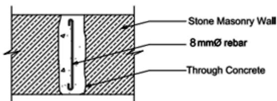
Fig. 12. Through wall concrete in an existing SMM wall
