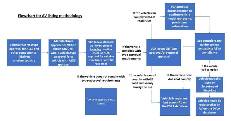
The flowchart for AV listing methodology shows the process for how a decision is made to list a vehicle equipped with ALKS. It explains that a vehicle must submit their vehicle to VCA to be considered for listing, and, if successful, is listed by Secretary of State on the recommendation of the VCA.
