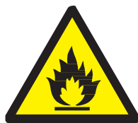
Flammable material or high temperature 1
