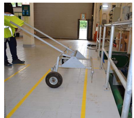
Image 3.5 Purpose built lifting and handling cart for lifting and handling heavy covers
