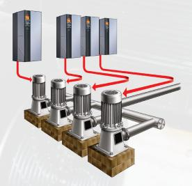
A typical VLT®AQUA Drive installation utilizing the Cascade Controller option via MODBUS in conjunctionwith three additional VLT®AQUA Drives to operate one to four pumps as demand requires.
