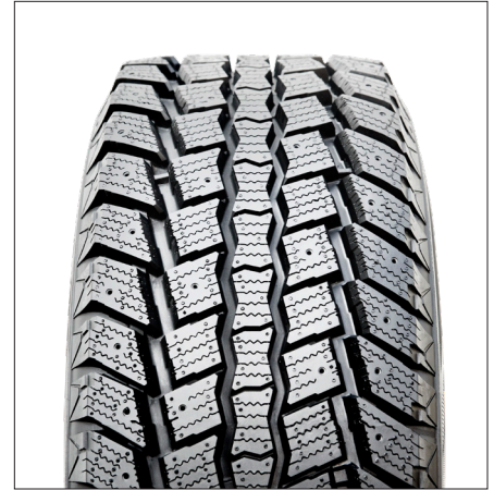
The WST2 features a zigzag sipe arrangement engineered for excellent directional grip on snow and ice, while its angled grooves effectively evacuate slush and water.
