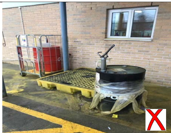
Incorrect storage of oil barrels on ground and improper use of York
